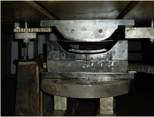
Fig. 12. Schematic diagram of stamping die assembly.
