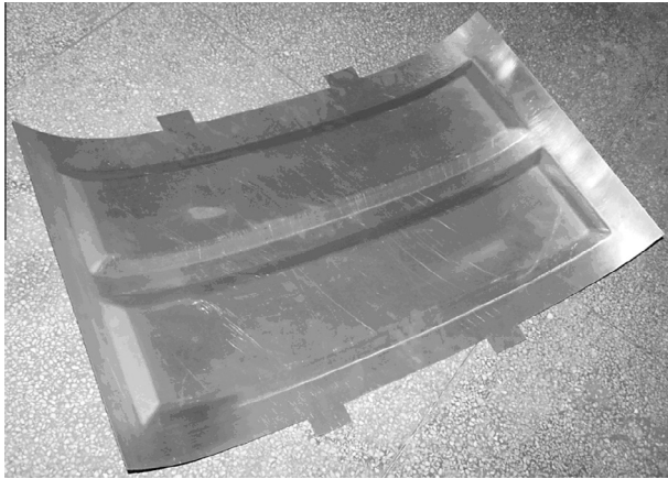
Fig. 19. The aircraft skin part manufactured in the factory.
