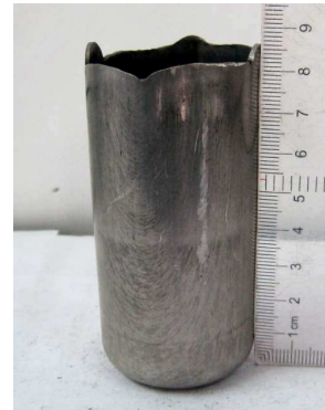
Fig.3 The effects of temperature on LDR Fig.4 The cylindrical cup of 80mm in height The effect of drawing temperature on the microstructure of drawn cup walls The microstructures of drawn cup walls at 403K, 423K, 443K and 473K were shown in Fig.5.
